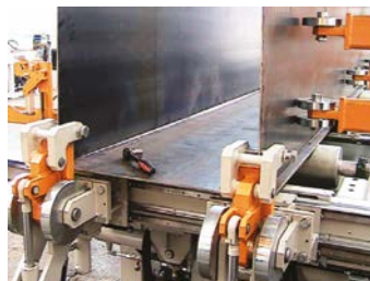
Double Edge Tack-welding unit
