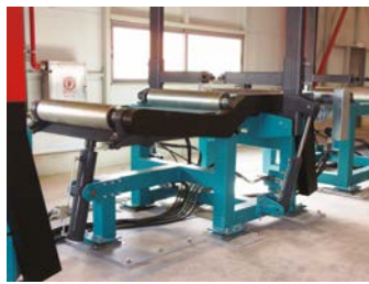
Infeed roll for camber
